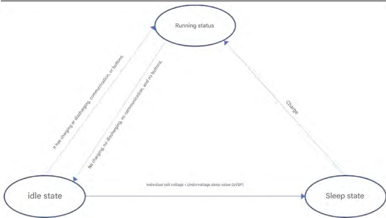
Operating modes for unmanned flight scenarios are divided into flight and non-flight states. While in flight, the battery does not provide any discharge protection (such as undervoltage or high discharge temperature); only warnings are reported. Once flight mode ends, if these issues persist, battery protection activates immediately. Note: During flight, the short press + long press shutdown feature is disabled.
